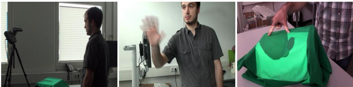
**Fig. 2.** (left to right) Coupled projector-Kinect device where visual data is projected on interaction zone (green sheet); user initiates tracking with hand wave gesture; pinch-and-pan gesture to interact with the projected virtual information on a curved surface.
